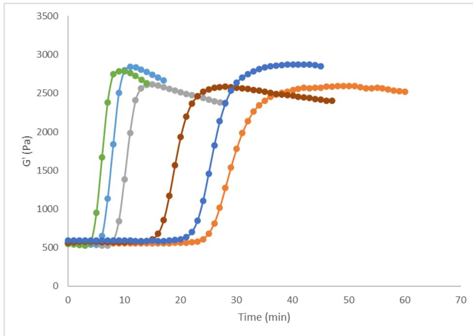
Figure 1. Viscoelasticity graphs for TeloCol 3 at Temperatures: (green) 37°C taken day 1, (light blue) 30°C taken day 1, (gray) 25°C taken day 2, (red) 22°C taken day 3, (dark blue) 20°C taken day 1, (orange) 20°C taken day 2.
